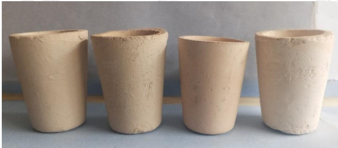
Figure 1: Photographs of the Fired refractory Crucible Samples
