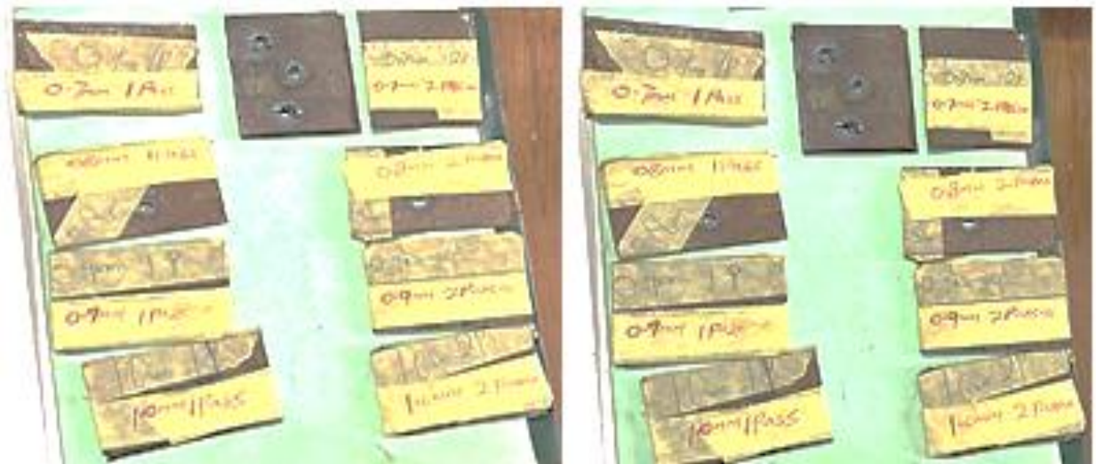
Fig. 2: Spot-welded Samples for Macroprofile and Microstructure Tests
