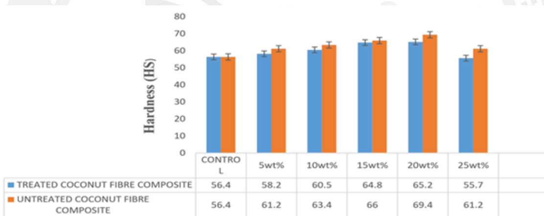
Fig. 5: Hardness Value of the developed composite and Control Sample
